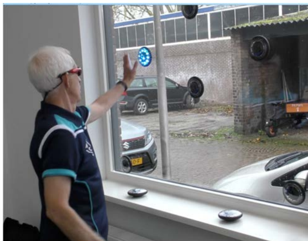
Figure 2. FitLight ® s mounted on a window for testing reaction time. The specification of the experimental set-up is in Appendix A.
